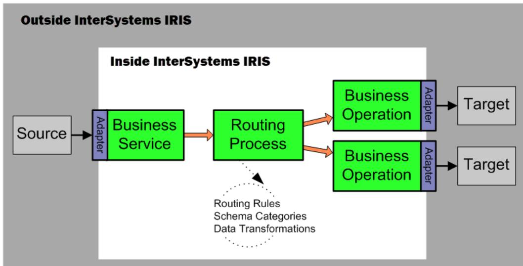
The following figure expands the diagram of a routing process to show how it uses routing rules to direct the flow of information through the interface. The following figure includes details about the routing rules and data transformations that are only implied by the dotted circle in the diagram above.
